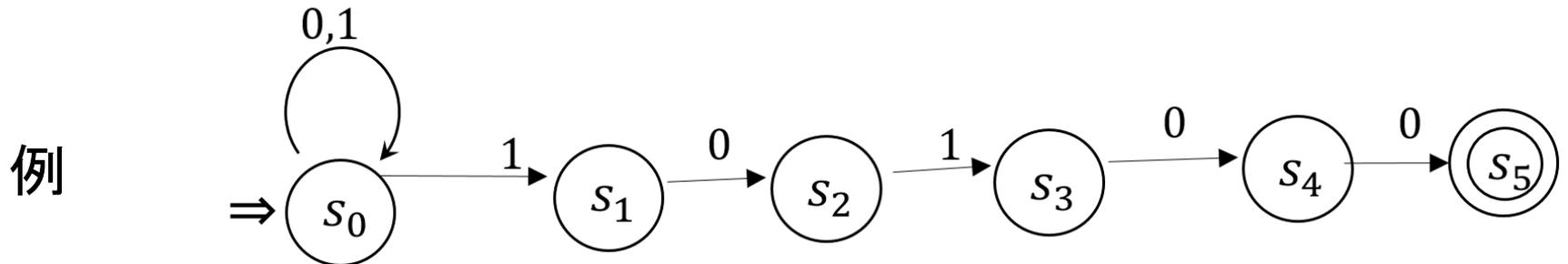
$$\delta'(s_0, 101) = \{q \in K \mid \exists p \in K (p \in \delta'(s_0, 10) \wedge q \in \delta(p, 1))\}$$
